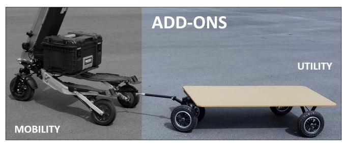
Utility can be added to the vehicle in multiple ways, without compromising the personal mobility aspect. A cargo box, a toolbox, an EMS kit or a trailer that can be quickly connected to the Trikke vehicle to move supplies, tools, parts, packages, rescue and medical gear.
