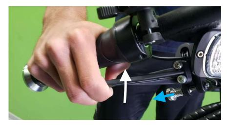
**UNLOCK** 1- squeeze brake lever
