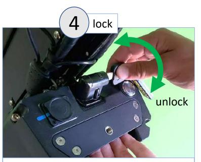
Lock the battery by turning key 90 degrees CW – **remove the key!**
