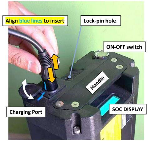
\* Battery can also be charged while mounted to the vehicle
