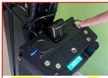
**WARNING** Switch battery **OFF** For removal and installation
